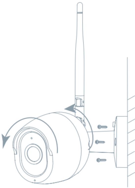
1. Fix the Camera to the wall with screws
